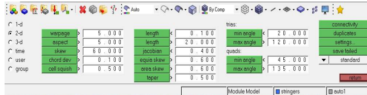
Figure 4.5: Elements checking in hyper mesh
